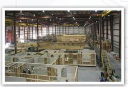
At the first station, two people build a floor section. "They buy only the best lumber available", says one of the workmen, "then we don't have to spend time culling out poor lumber." One is reminded they exclusively use kiln dried lumber (they even test the moisture content on each delivery) so the frame of the house won't be subjected to shrinking or twisting. Vast quantities of glue are used in addition screws, nails and bolts.
